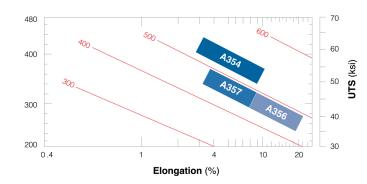
This figure compares the quality index achievable with VersaCast versus the common casting alloys A356 and A357. This plot shows the strength of rapidly solidified, permanent mold castings. Constant values of the quality index are shown by red lines.
