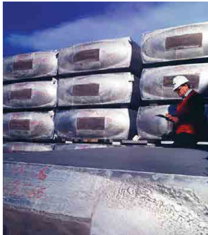
Much of the smelter's metal was cast into slab before being rolled to customer specification. Photo by Peter Garside.
