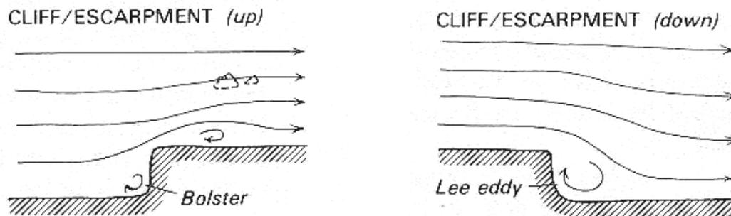
Figure 44: Typical patterns of airflow over an escarpment (from Oke, 1987).
