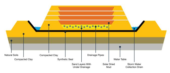
Figure 7-3: Schematic showing construction method of residue drying beds.
