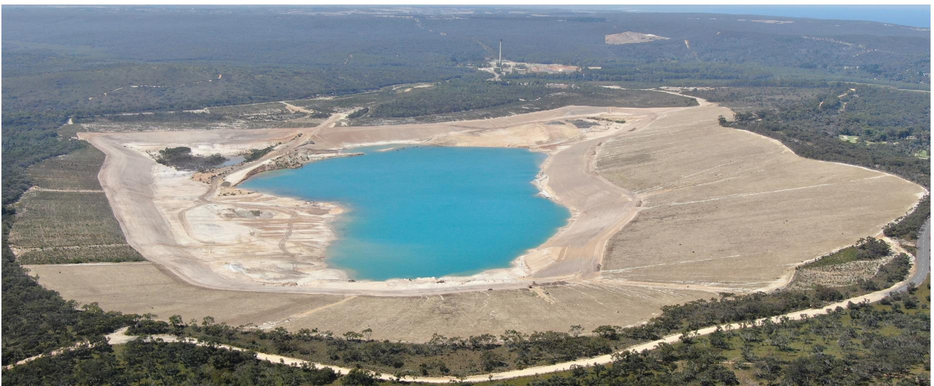
Above: A view of the mine looking east towards the power station site. The current water level is RL -16.3 metres, representing approximately 18 per cent of the proposed full volume.
