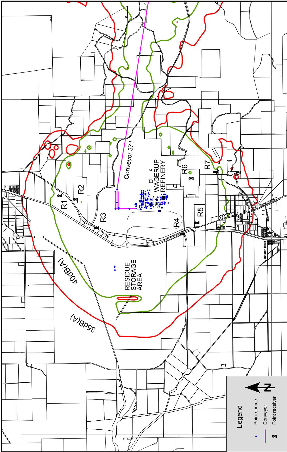
Figure C1. Noise Contours for Expanded Refinery - With Noise Control.
