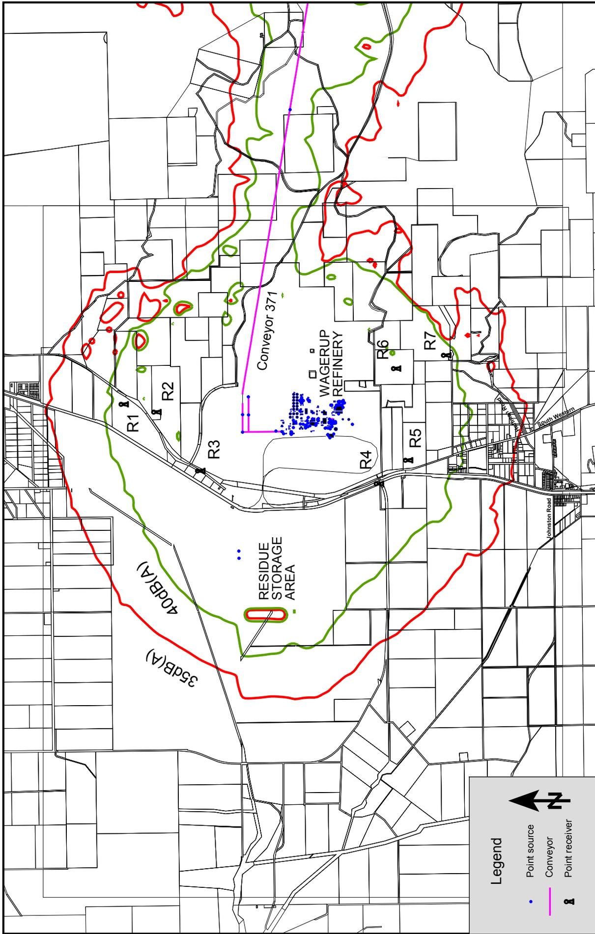
Figure A1. Noise Contours for Existing Refinery
