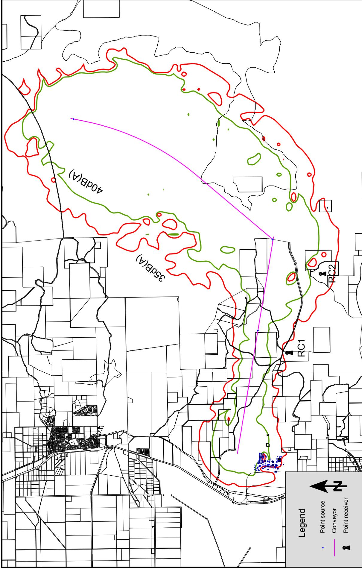
Figure A2. Noise Contours for Existing Overland Conveyors.
