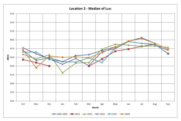
Figure 6-3 Comparison of noise levels measured at Location 2 (South Monitor) for base period (2002 – 2003) and 2014 – 2018
