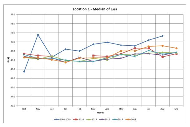
Figure 6-2 Comparison of noise levels measured at Location 1 (North Monitor) for base period (2002 – 2003) and 2014 – 2018
