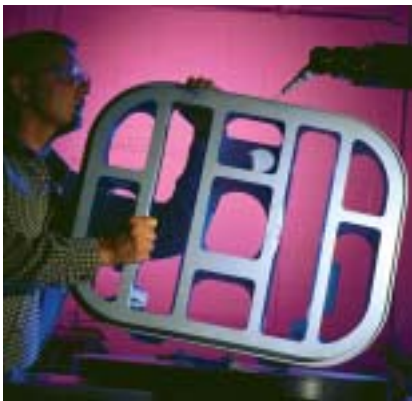
Large, complex, asymmetrical castings consolidate multiple details in a single piece and can cut costs at every step from initial design through production and inspection.
