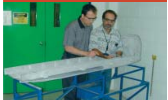
Sylvain Poissant (left), general manager of Laval Casting, inspects a large, structural casting for dimensional accuracy. Laval specialises in large, high-property aerospace castings.
