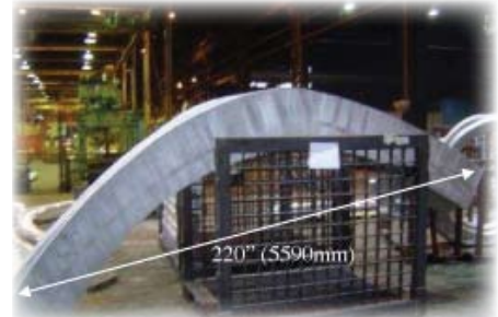
Example of a large contoured hand forged product produced for the aerospace industry.
