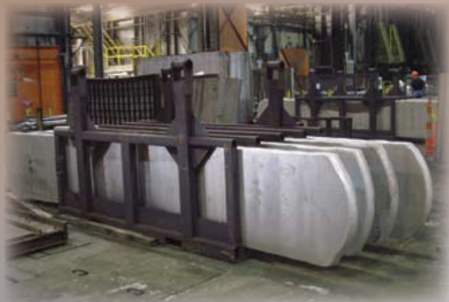
144" x 48" x 7" SSR ™ Forged Billet replacement for Boeing commercial aircraft.
