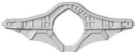
CTOL 450 bulkhead, 18 x 6.5 ft
