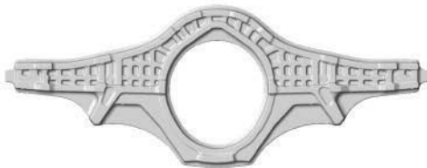
CTOL 472 bulkhead, 19.5 x 6.5 ft
