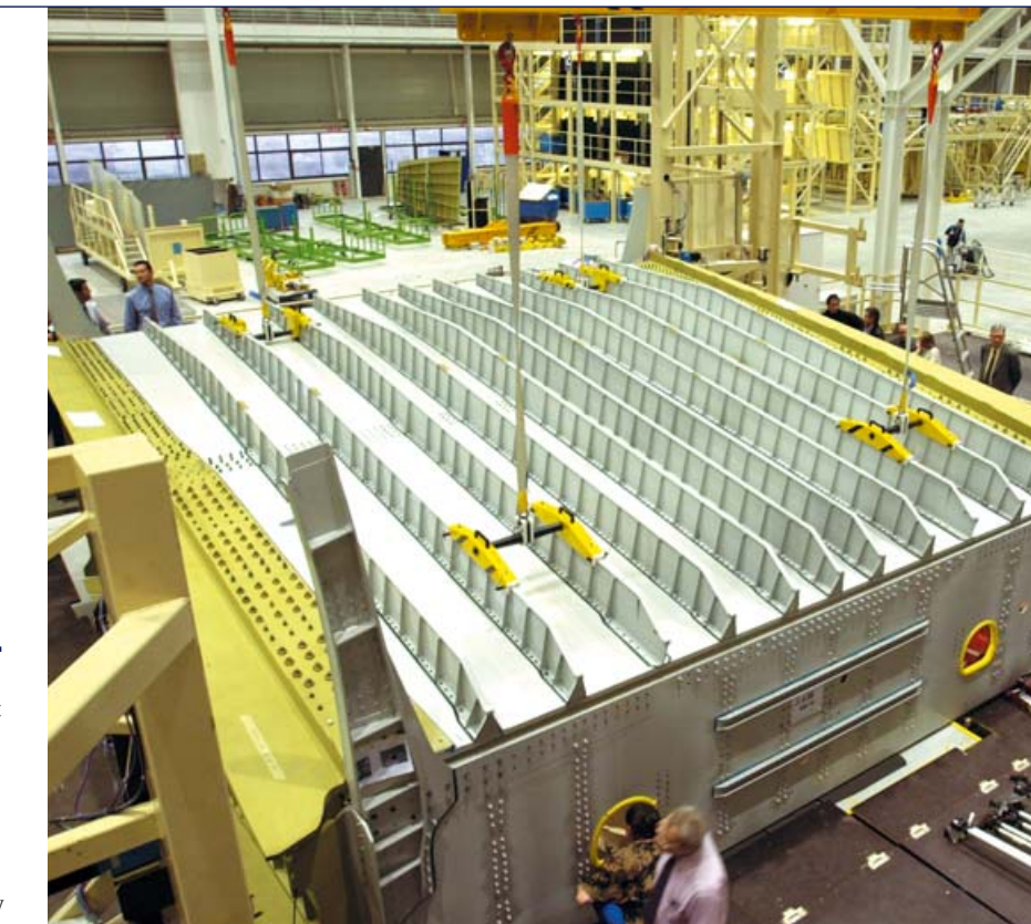
▲ The A380's center wing box is the largest composite component in aviation history and for the first time, the rear fuselage section immediately behind the pressure bulkhead is also being produced using composites.
