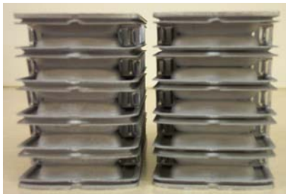
With I/L (no skips at 6 g/m 2 ) No I/L (numerous leaks at 10 g/m 2 )
