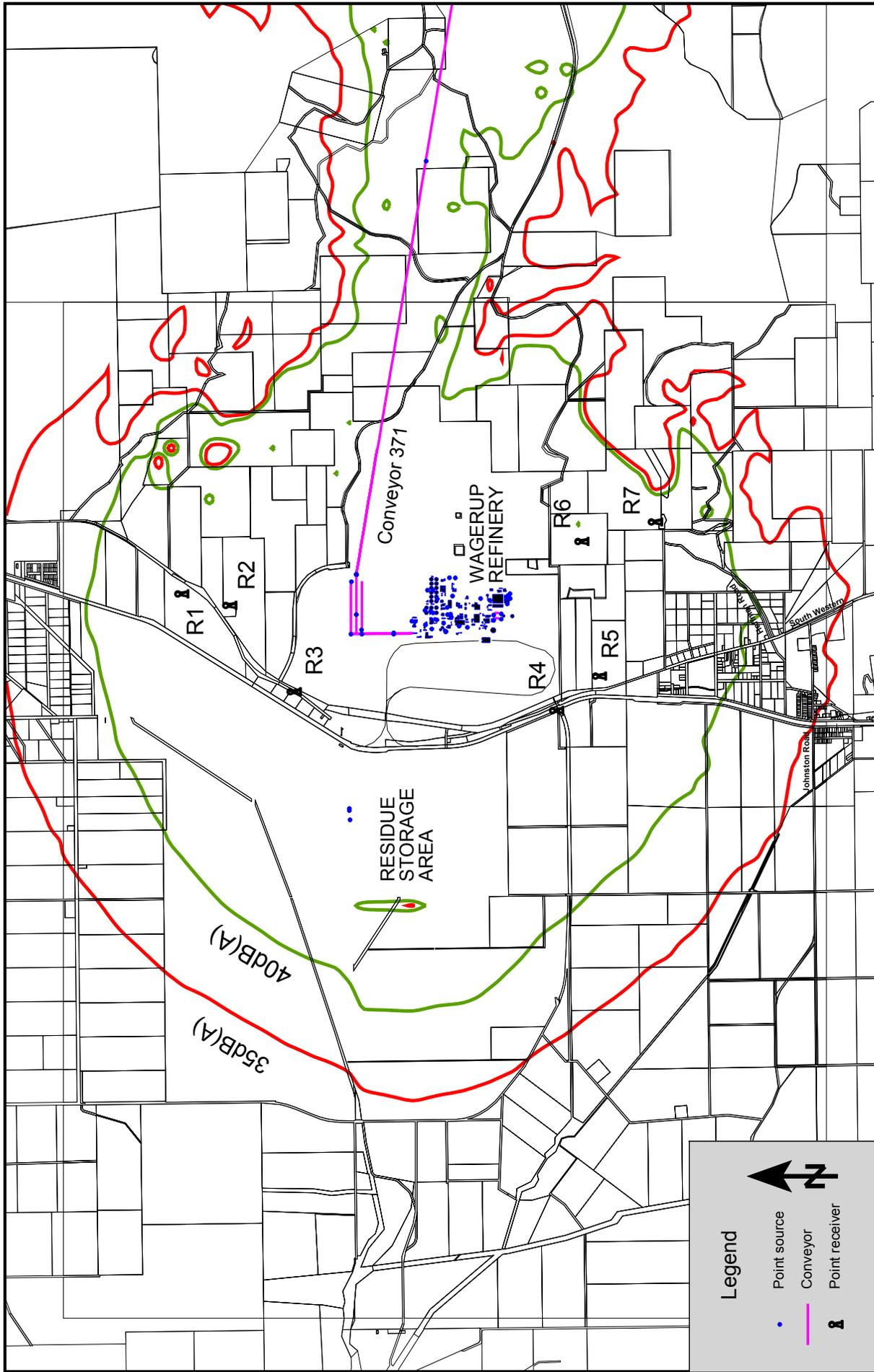
Figure B1. Noise Contours for Expanded Refinery - Without Noise Control.
