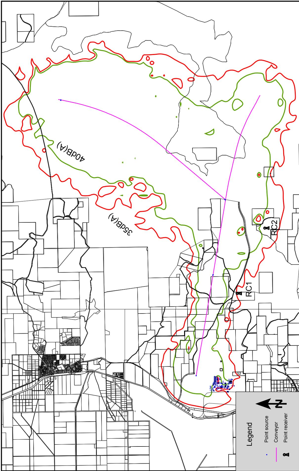
Figure B2. Noise Contours for Expanded Overland Conveyors - Without Noise Control.
