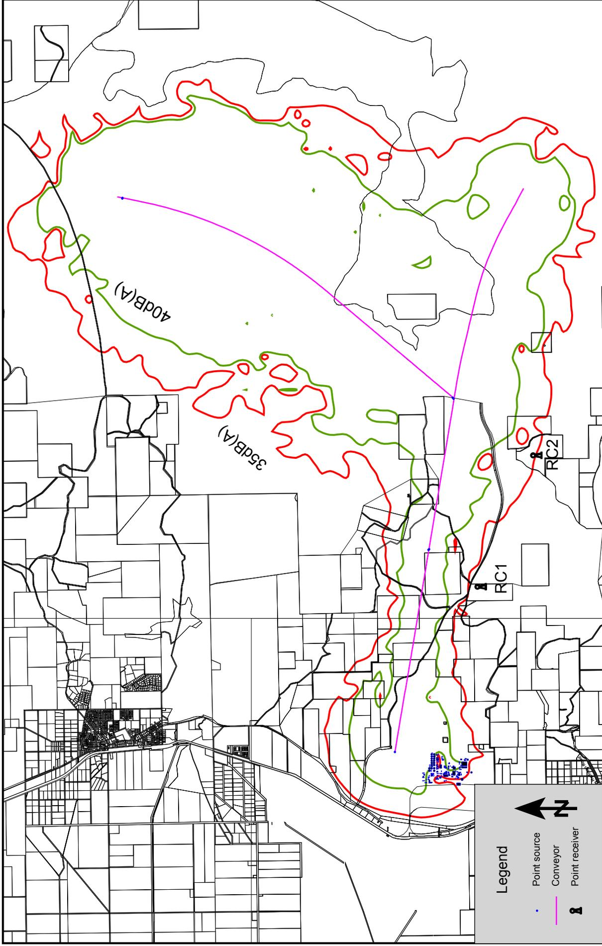
Figure C2. Noise Contours for Expanded Overland Conveyors - With Noise Control.
