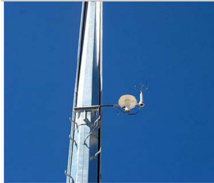
Figure 23: 10-m wind sensor at Bancell Road (from SKM, 2003).
