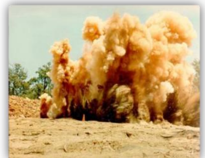
The caprock layer is blasted to access the bauxite beneath it
