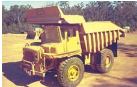
One of Huntly's first fleet - CAT 769B with a payload of 35 tonnes
