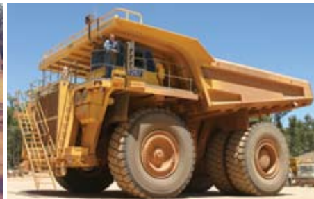
Huntly's latest fleet - Komatsu 730E haul truck with a payload of 190 tonnes
