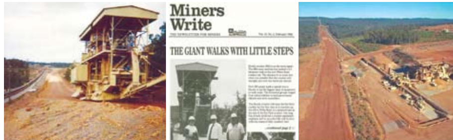
Crusher No.2 walking from North Road to the White Road crusher site
