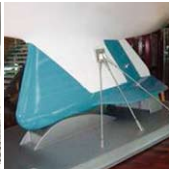
The winged keel of Australia II, developed in 1983
