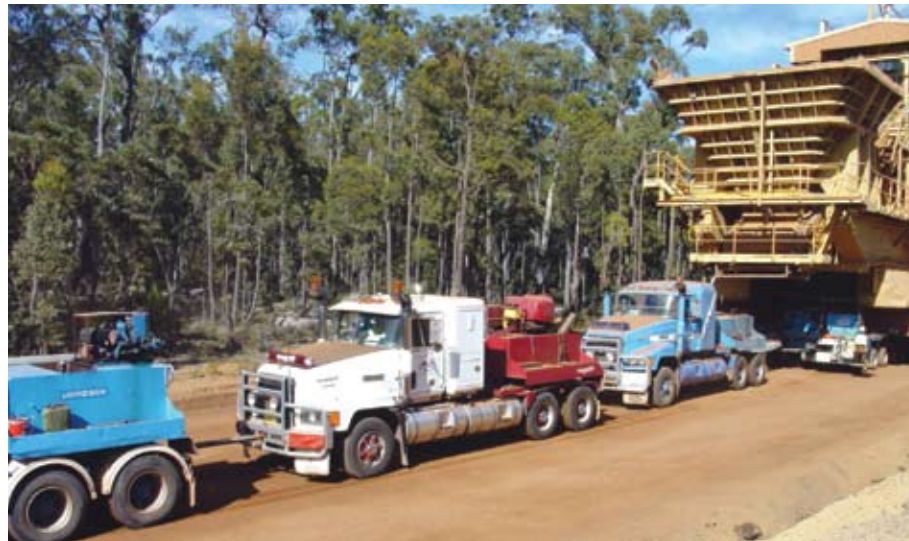
160 crusher on a low loader being pulled by three semi-trailers in August 2004
