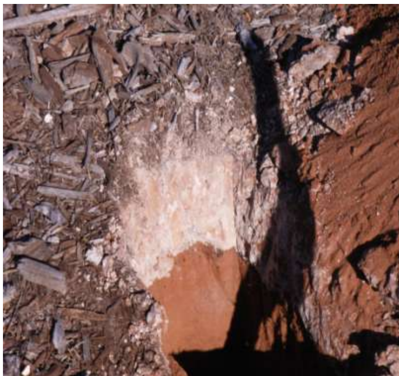
Figure 7. (a) Large pieces of gypsum present within the residue sand profile, and (b) high concentrations of gypsum in the 0 – 200 mm depth interval at the shallow gypsum incorporation trial.
