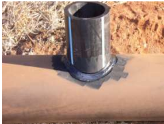
Figure 17. Sump drain pipe constructed from polypipe with connectors for receiving draincoil
