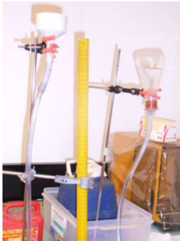
Figure 7. (a) Pressure plate apparatus and (b) hanging-water column equipment used to construct moisture characteristic curve for residue sand
