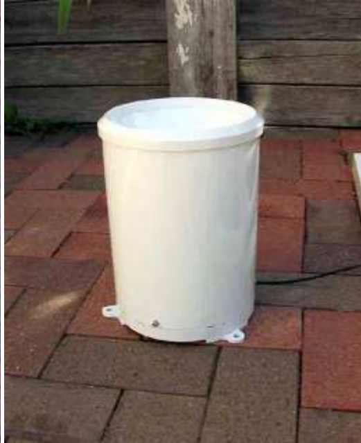
Figure 31. (a) Complete weather station, (b) SL5-1 smart logger and IB14 databus hub in waterproof enclosure (c) TA1 Air temperature sensor and HU1 Relative humidity sensor, (d) Sensor shelter that allows air through flow but not direct sunlight, (e) WD2 Wind direction sensor, SR2 Solar radiation sensor and AN2 Anemometer, and (f) Tipping bucket rain gauge
