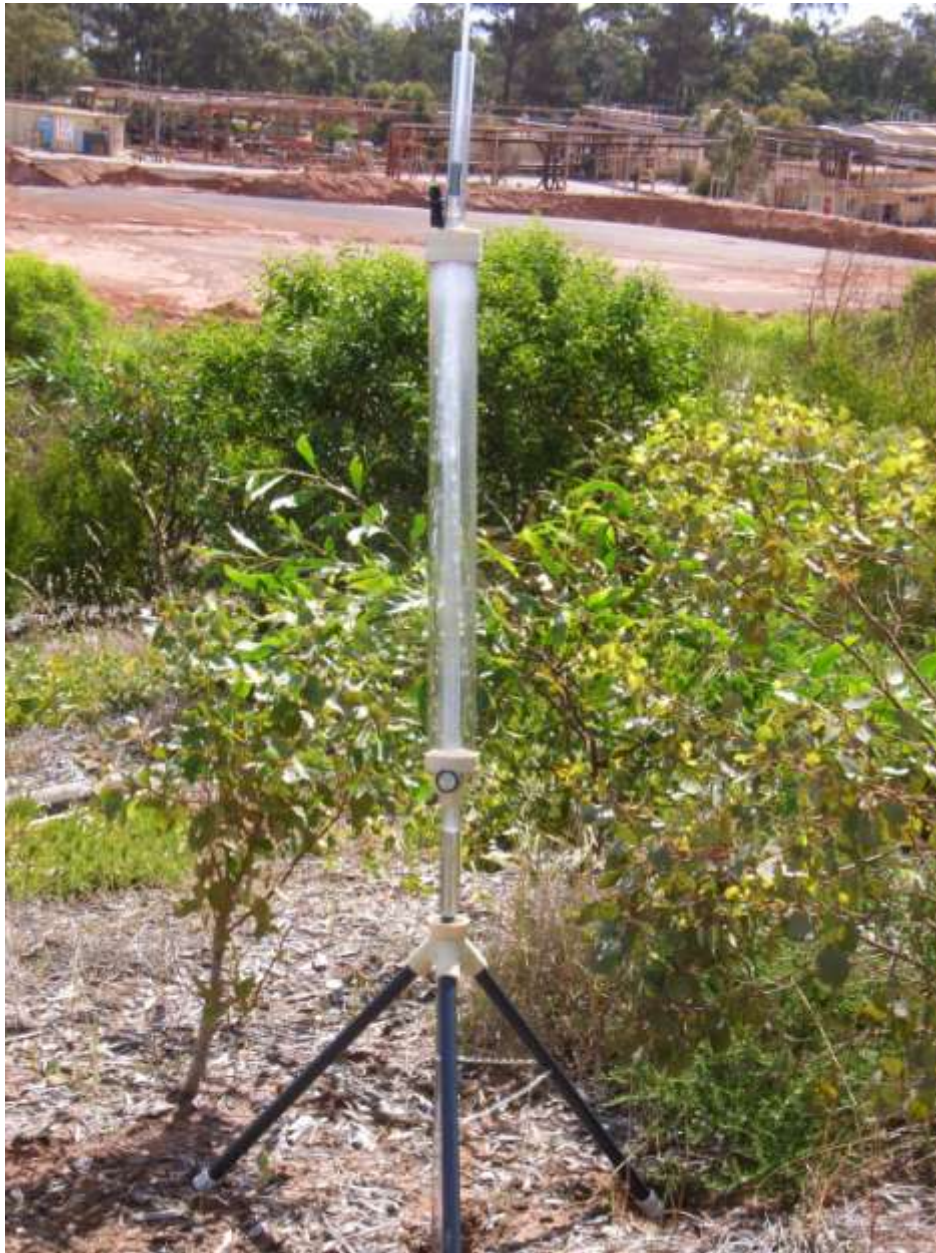
Figure 6. Guelph constant head permeameter used for measuring saturated hydraulic conductivity within residue sand profile
