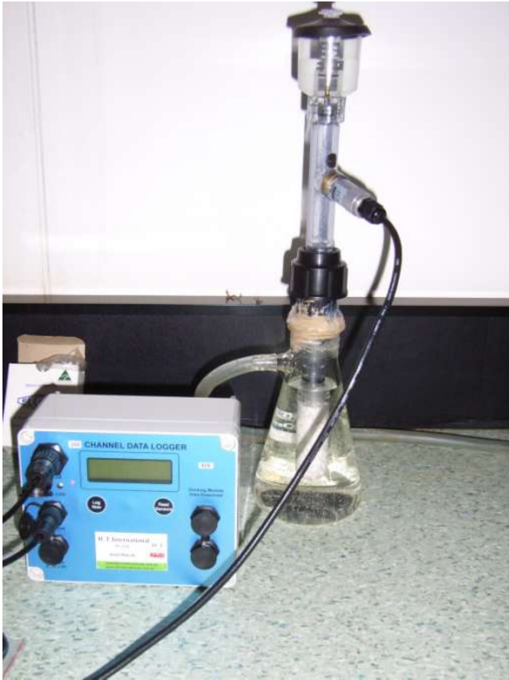
Figure 8. Jet-fill tensiometer fitted with pressure transducer for monitoring in-situ pore-water tension within residue sand profile
