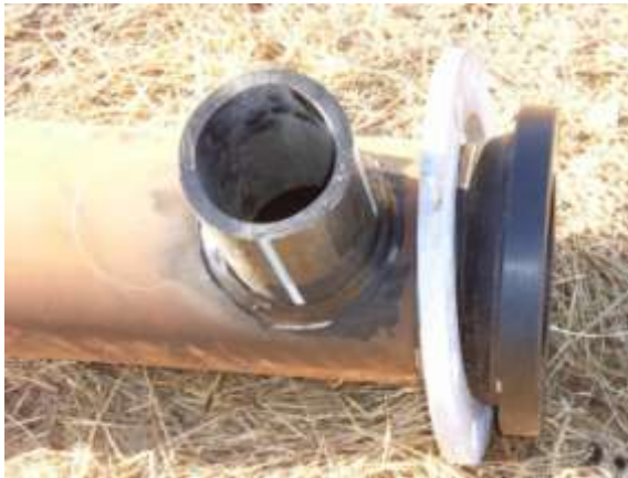
Figure 17. Sump drain pipe constructed from polypipe with connectors for receiving draincoil
