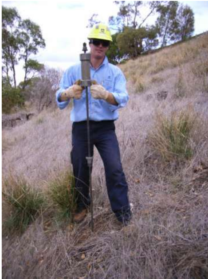
Figure 5. Perth sand penetrometer used for measuring penetration resistance within residue sand profile
