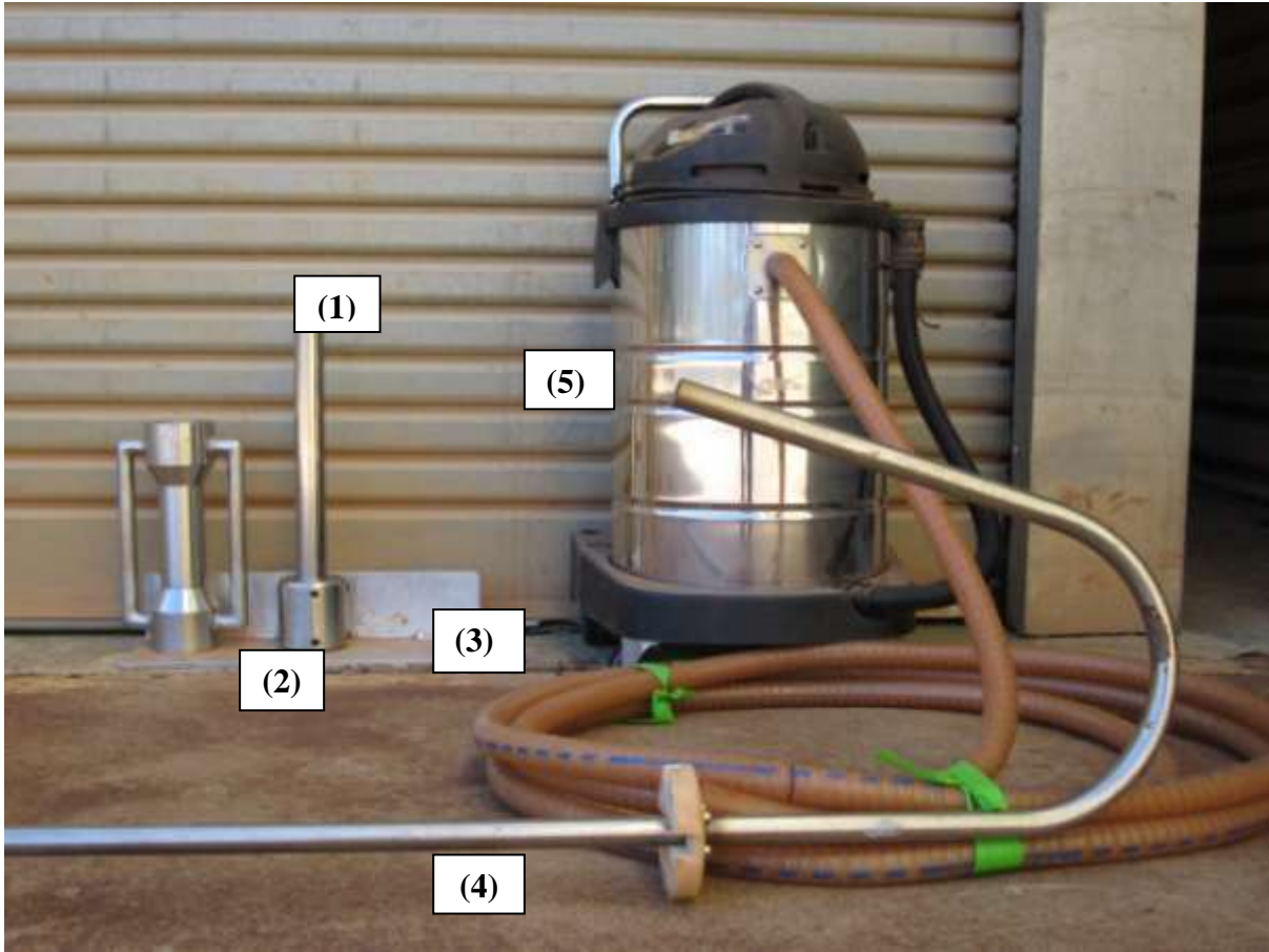
Figure 1. Essential equipment required for installing neutron probe access tubes in residue sand profiles. (1) the stainless steel tube, (2) an anvil and slide hammer, (3) a base plate for locating the tube, (4) a sand extraction tube, and (5) an industrial vacuum cleaner and vacuum hose.
